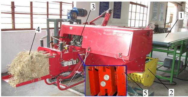
**Figure 4.** Straw square bales compression and baling test rig. 1, material conveyor; 2, straw pickup mechanism; 3, knotting device; 4, straw square bale; 5, pressure straw piston.
