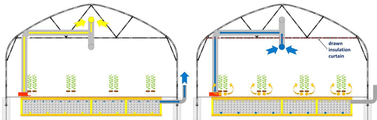
**Figure 1.** Charging the heat accumulator during a warm day (left) and discharging the accumulator for plant heating during the night or cold day (right).
