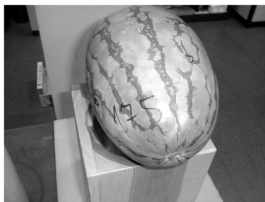
Figure 1. Structural elements of the impact acoustic response device. Left: diagram showing the structural elements and microphone. Right: watermelon awaiting excitation at an equatorial point.
