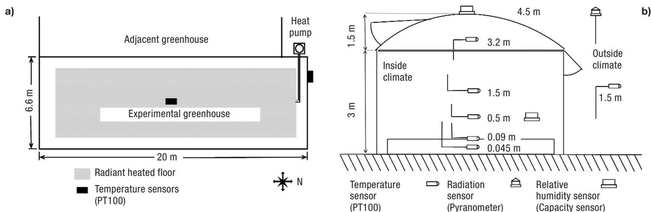
**Figure 1.** a) Plan view of the experimental greenhouse; location of the heated floor and the air-water heat pump. b) End view of the experimental greenhouse with the sensor system.
