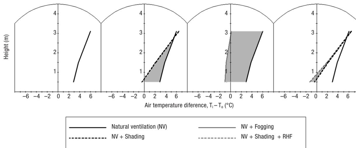
**Figure 5.** Experimental data: mean values for the critical period 13:00-17:00 h. Graph comparing the air temperature difference obtained from different cooling strategies, T<sub>i</sub> - T<sub>o</sub> (°C) at different heights. The shaded area shows the improvement of the cooling effect achieved with the addition of technologies.
