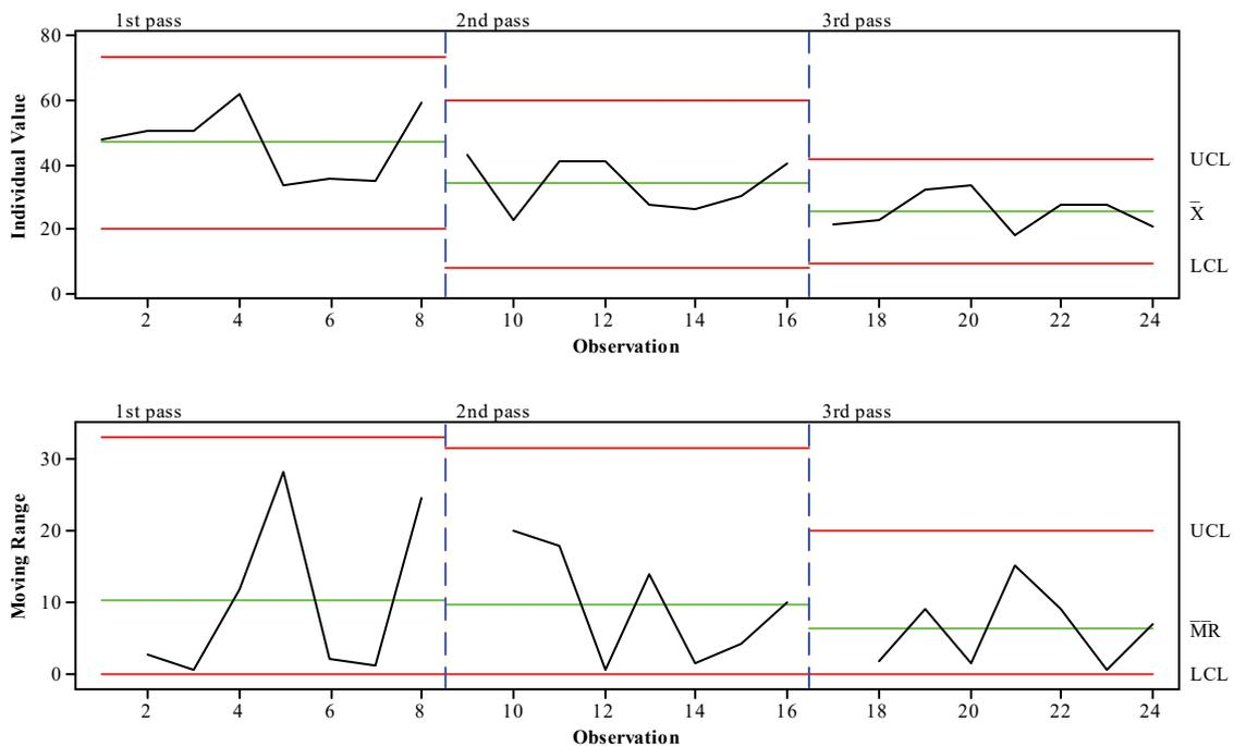
Figure 4. Control chart of individual values of cleaning efficiency (%).
