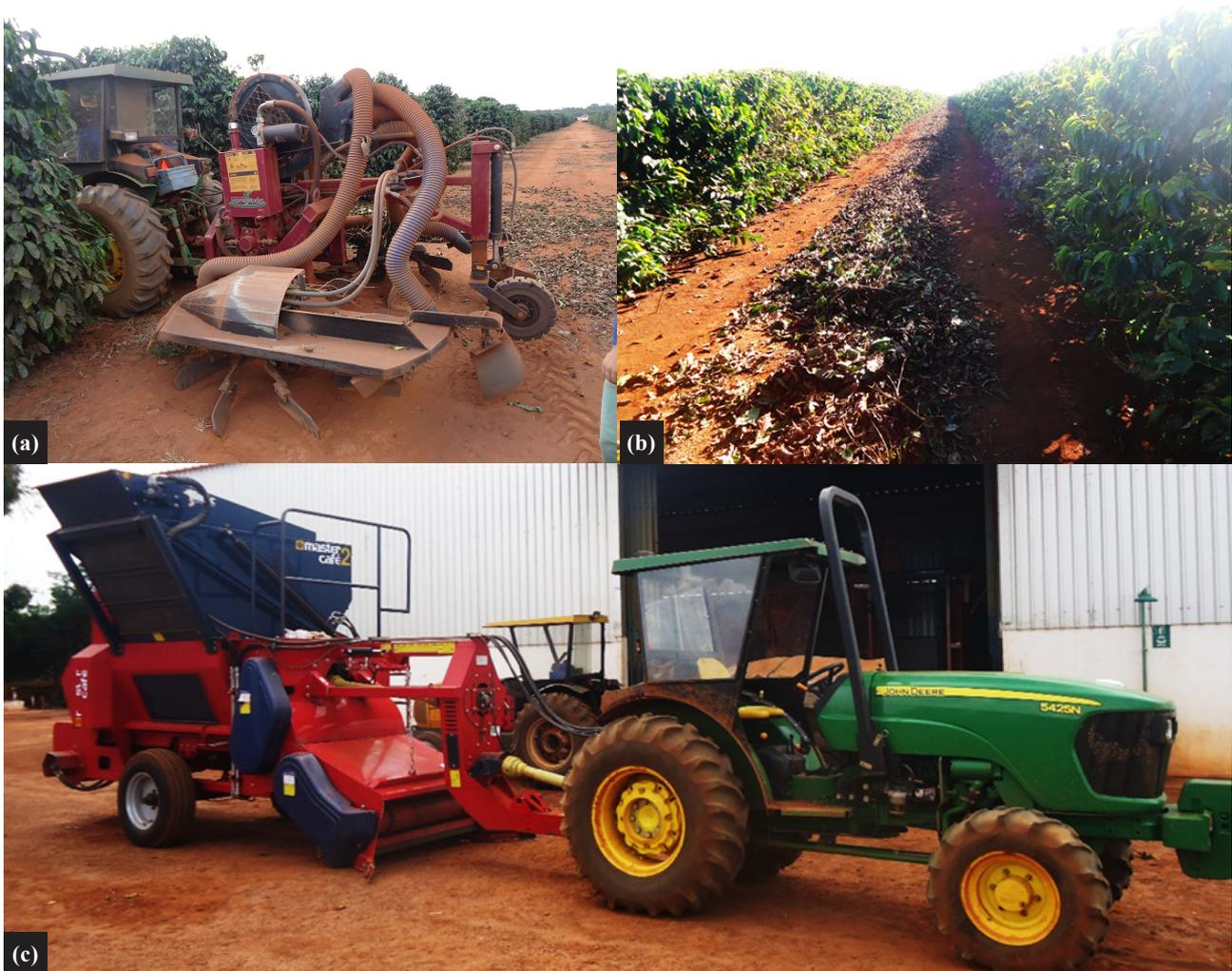
**Figure 1.** Mogiana mounted sweeper-blower (a); coffee and impurities joined at the center of the interrow, ready for the picking operation (b); MIAC Master Café II picker machine for mechanized picking (c).
