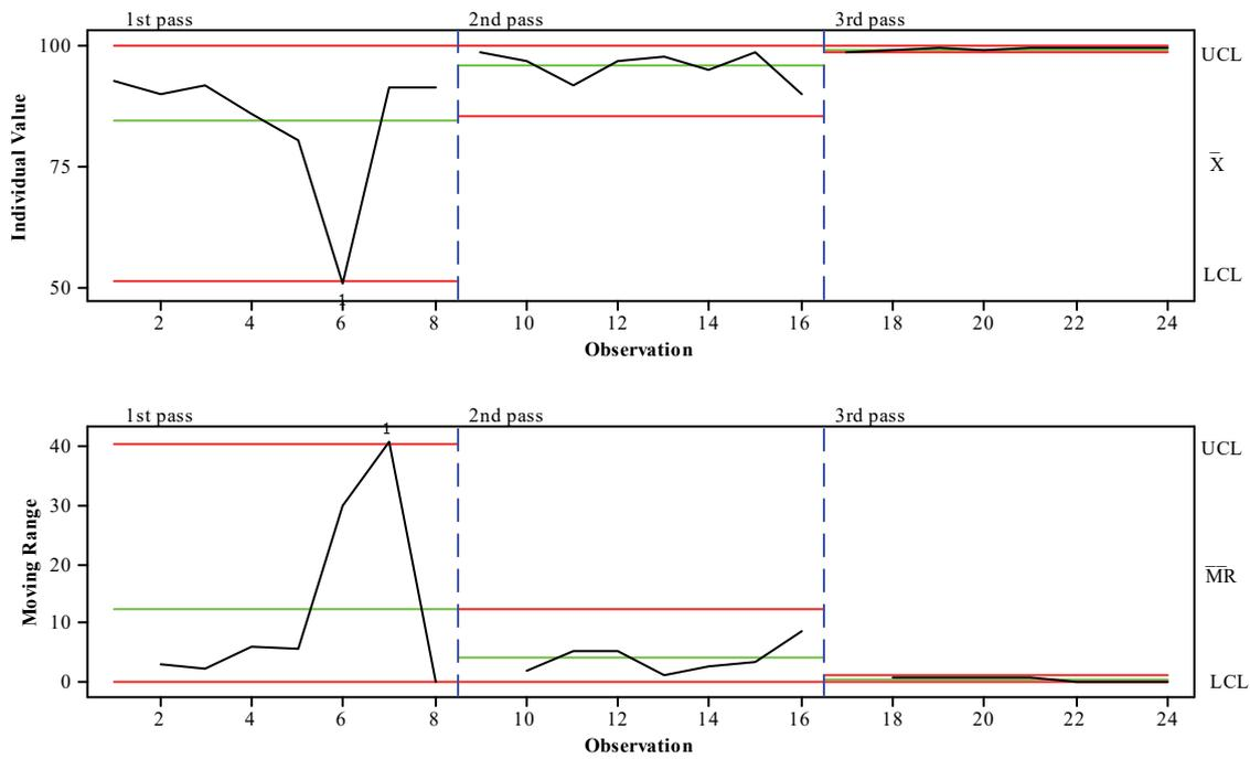
Figure 3. Control chart of individual values of picking efficiency (%).
