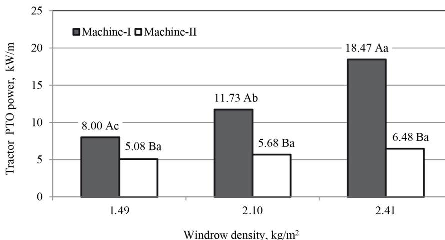
**Figure 2.** PTO power requirements per working machine width. The different upper and lower case letters above the histogram bars indicate significant differences ( $p < 0.001$ , Duncan test) between the machines and the windrow densities, respectively.
