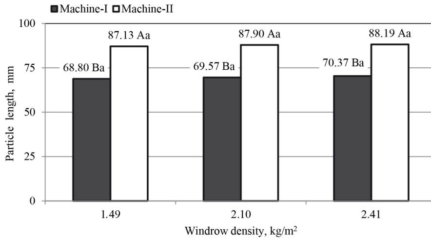
**Figure 3.** Lengths of the average particles. The different upper case letters above the histogram bars denote significant differences between the machines ( $p < 0.001$ ). The same lower case letters above the histogram bars denote non-significant differences among windrow densities at a probability of  $p < 0.05$ .
