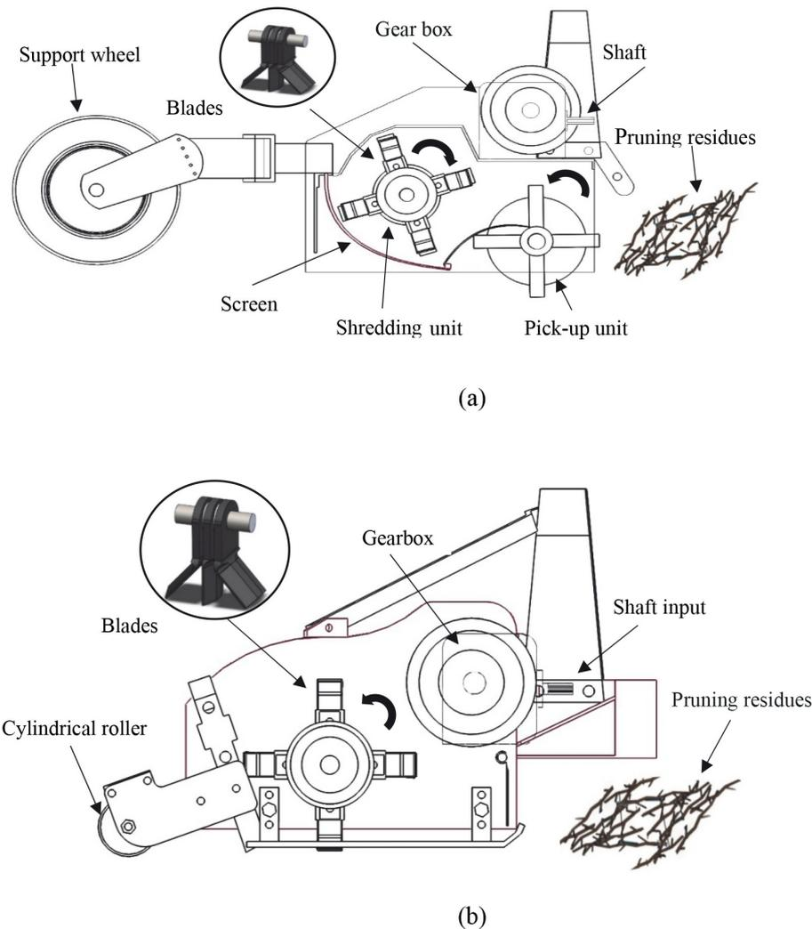
**Figure 1.** Schematic views of Machine-I (a) and Machine-II (b).
