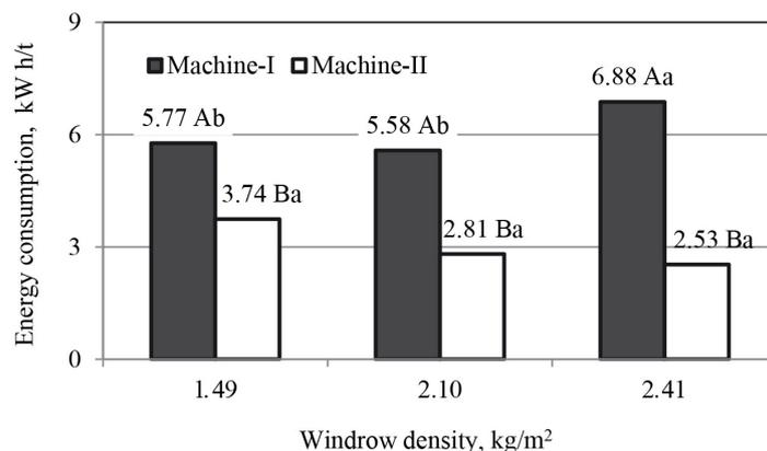
**Figure 5.** Energy consumption values per unit of shredded residue. The different upper case letters above the histogram bars denote significant differences between the machines at  $p < 0.001$ . The different lower case letters above the histogram bars denote significant differences between windrow densities ( $p < 0.05$ ).
