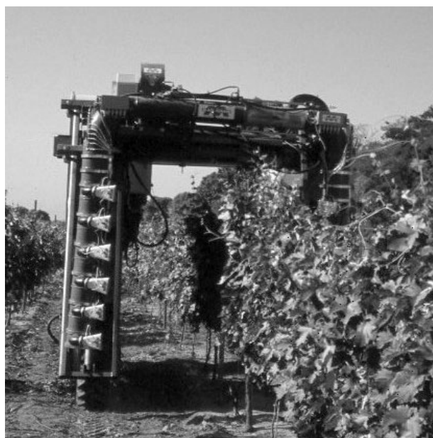
Figure 1. Rear view of the sprayer mounted on the over-the-row tractor.
