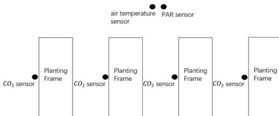
**Figure 4.** Scheme of the positions of the sensors used in the experimental greenhouse in the studied model.
