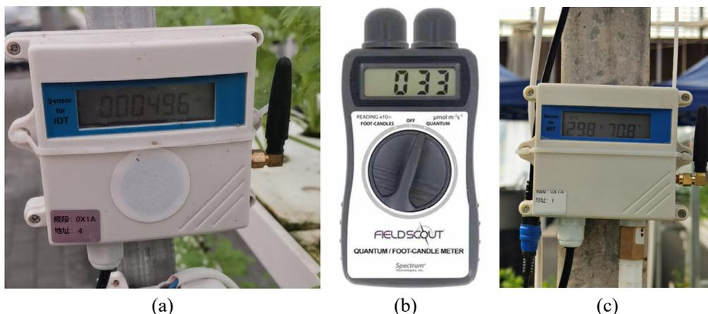
**Figure 3.** Sensors monitoring in the greenhouse located in Tongzhou, Beijing: (a) carbon dioxide concentration sensor; (b) photosynthetically active radiation sensor; and (c) air temperature and relative humidity sensors
