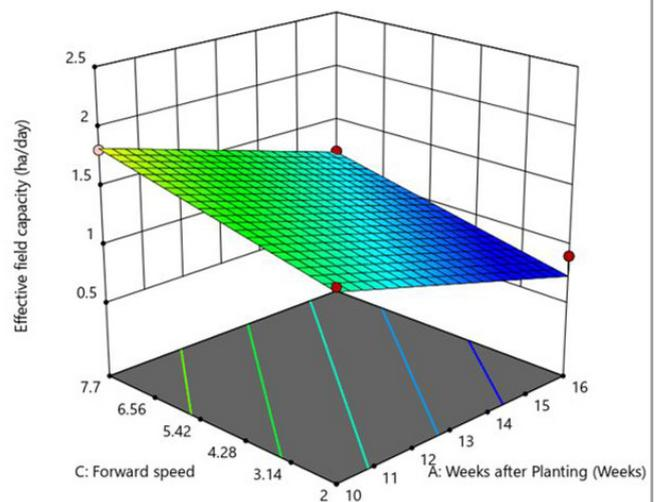
**Figure 3.** Effect of forward speed on effective field capacity of the machine.
