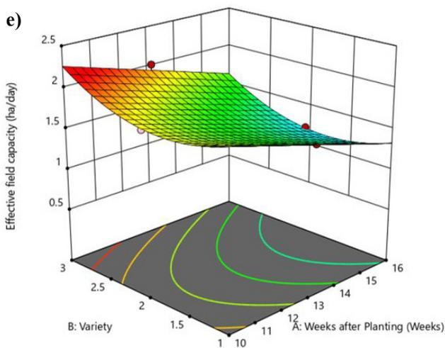
**Figure 2.** Effect of variety and weeks after planting (WAP) on effective field capacity when forward speed was (a) 2 km/h; (b) 3.5 km/h; (c) 5 km/h; (d) 6.5 km/h; (e) 7.7 km/h. Variety 1 = Cuba 108; Variety 2 = Ifeken Di 400; Variety 3 = Ifeken 400.
