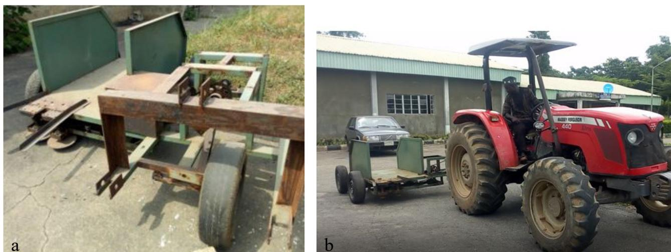
**Figure 1.** The fabricated kenaf harvester: (a) front view of the fabricated kenaf harvester; (b) the developed kenaf harvester mounted on a tractor.
