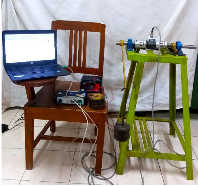
Figure S1. Torque transducer calibration.
