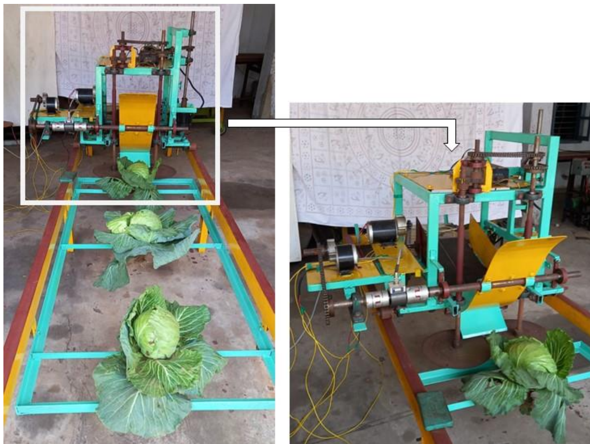
Figure S3. Laboratory experiment for measuring cutting and pushing torque.
