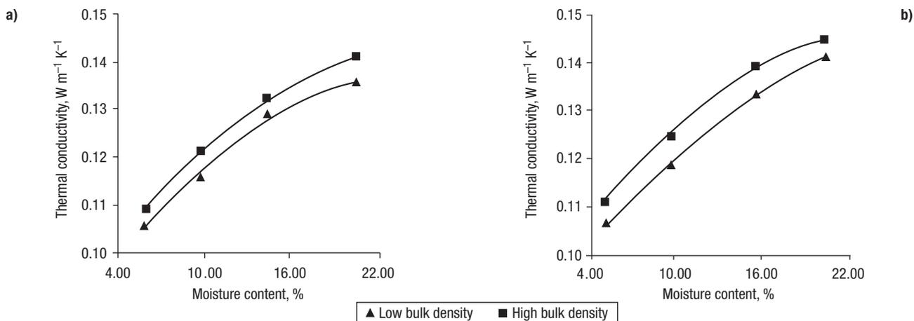
**Figure 3.** Thermal conductivity of safflower seeds at different moisture contents and two bulk densities for cv. Remzibey-05 (a) and Dinçer (b).
