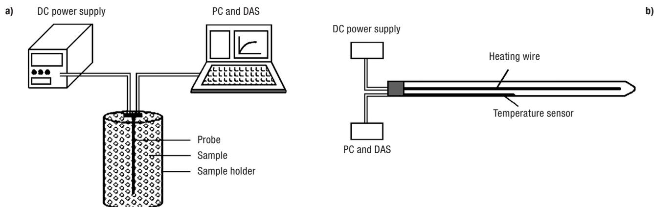
**Figure 1.** Thermal conductivity measurement system developed (a) and detail of the thermal conductivity probe (b). DAS: data acquisition system. DC: direct current.
