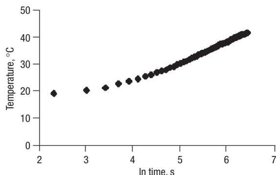
**Figure 2.** A typical thermogram showing the linearity of temperature *versus* ln time.
