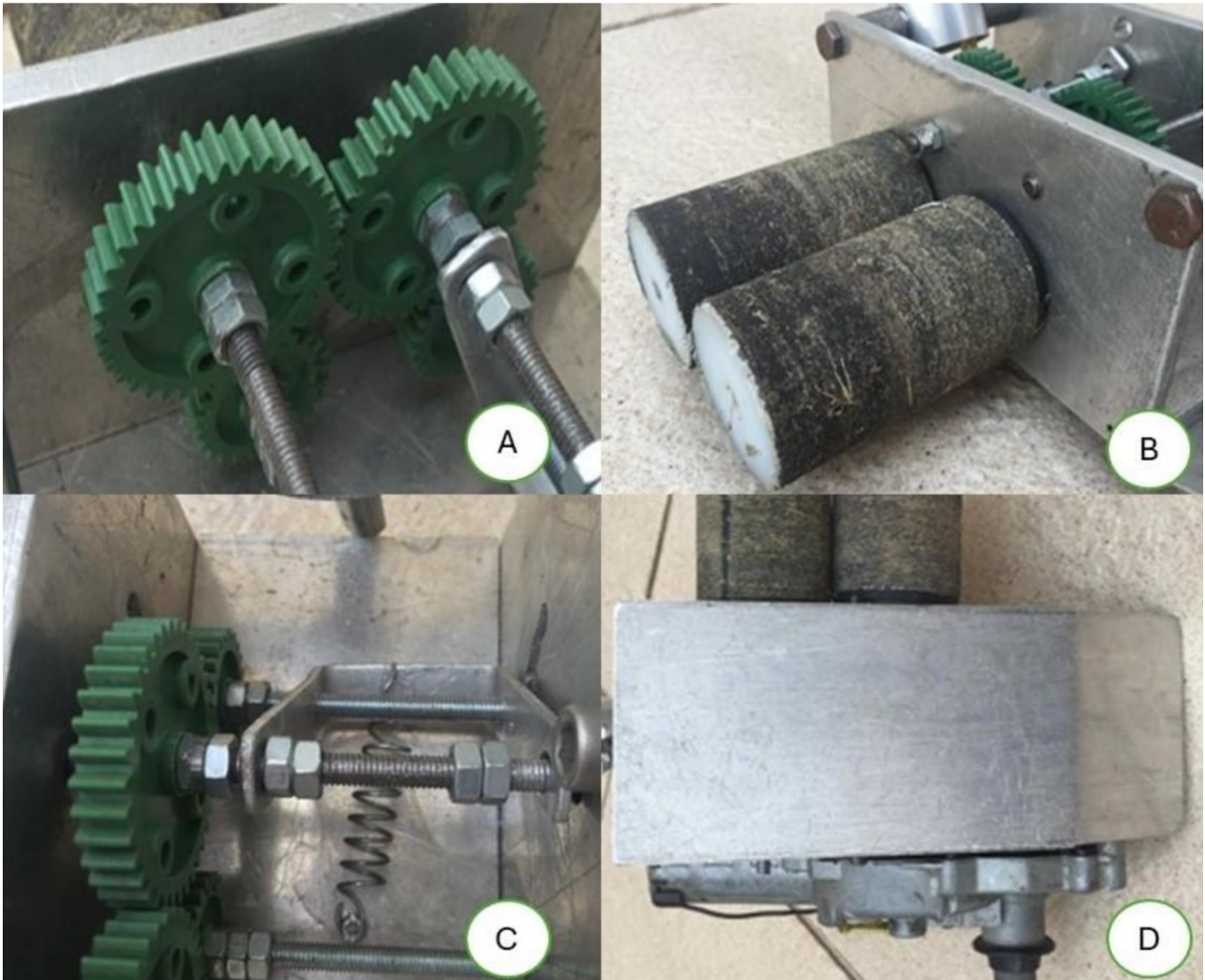
Figure 3. Transmission (a), removal (b), opening (c), and support (d) mechanisms built into the physical prototype.
