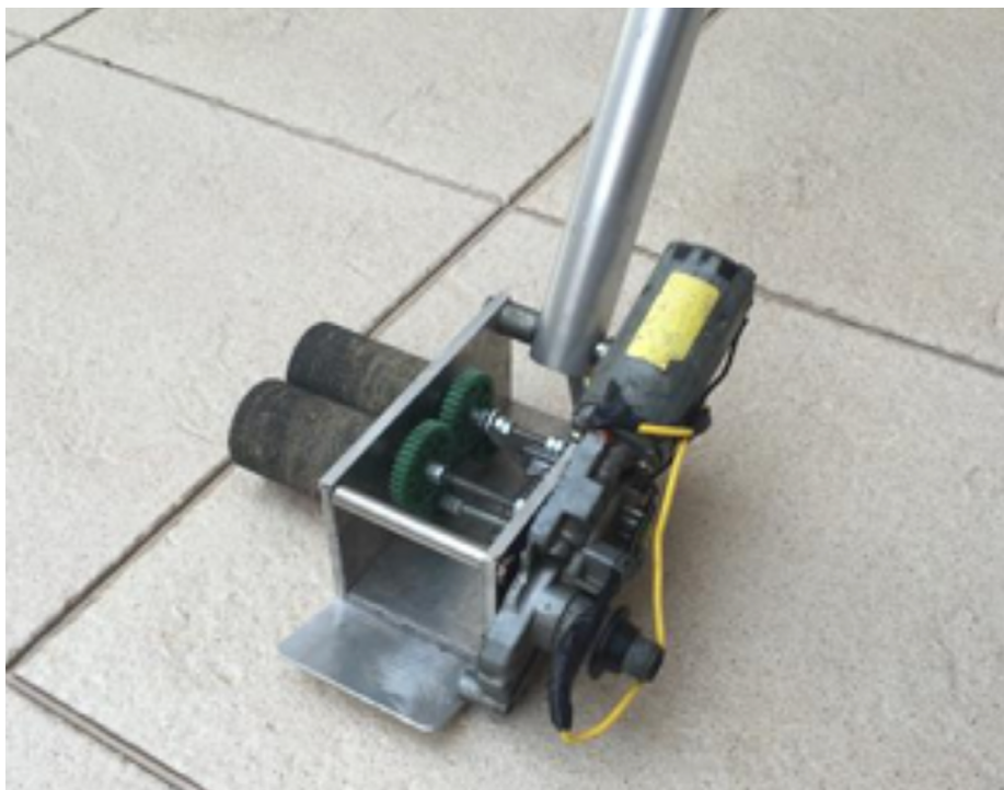
Figure 4. Physical prototype developed for mechanized weeding of vegetable beds.
