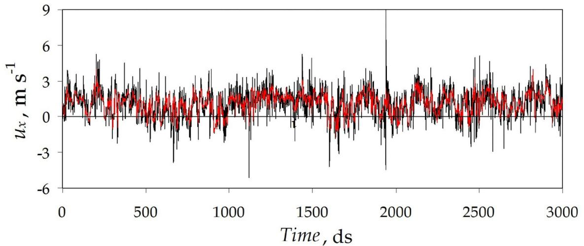
**Supplementary Figure 3.** Measurement using 3D sonic anemometers of the longitudinal component  $u_x$  over five minutes at the windward side vent. Experiment 2, inside surface of the vent (—); outside surface of the vent (—).
