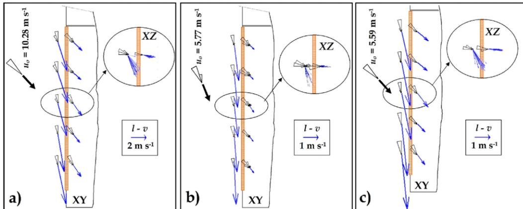
**Supplementary Figure 2.** Airflow diagram at the outside and inside surfaces of the northern side vent when facing windward. Experiments 4 (a), 6 (b) and 7 (c).
