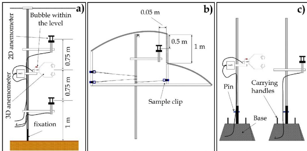
**Supplementary Figure 1.** Placement of the anemometers inside the greenhouse (a), at the roof vent (b) and outside the greenhouse (c).
