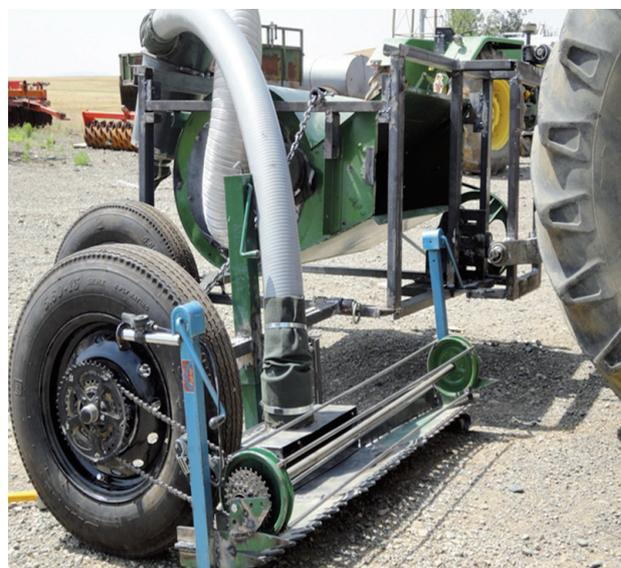
**Figure 8.** The tractor-mounted experimental harvester for chickpeas.
