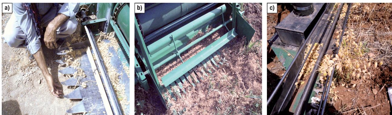
**Figure 3.** Physical models of the platform (a) and reel (b) for chickpea pod harvesting. Delivering performance of the reel (c).
