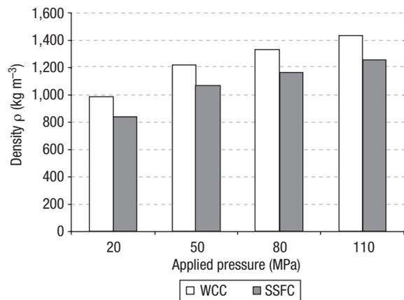
Figure 3. Average density values (kg m<sup>-3</sup>) of WCC and SSFC obtained using different pressure levels (20, 50, 80 and 110 MPa).
