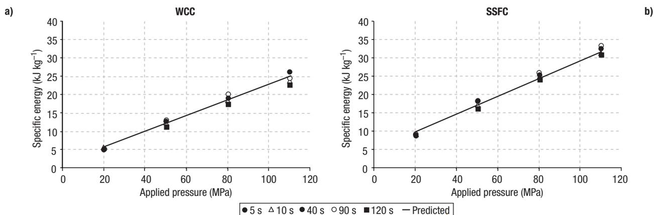
**Figure 4.** Relationship between applied pressure and specific compression energy to form the WCC (a) and SSFC (b) briquettes (pressure range 20-110 MPa).
