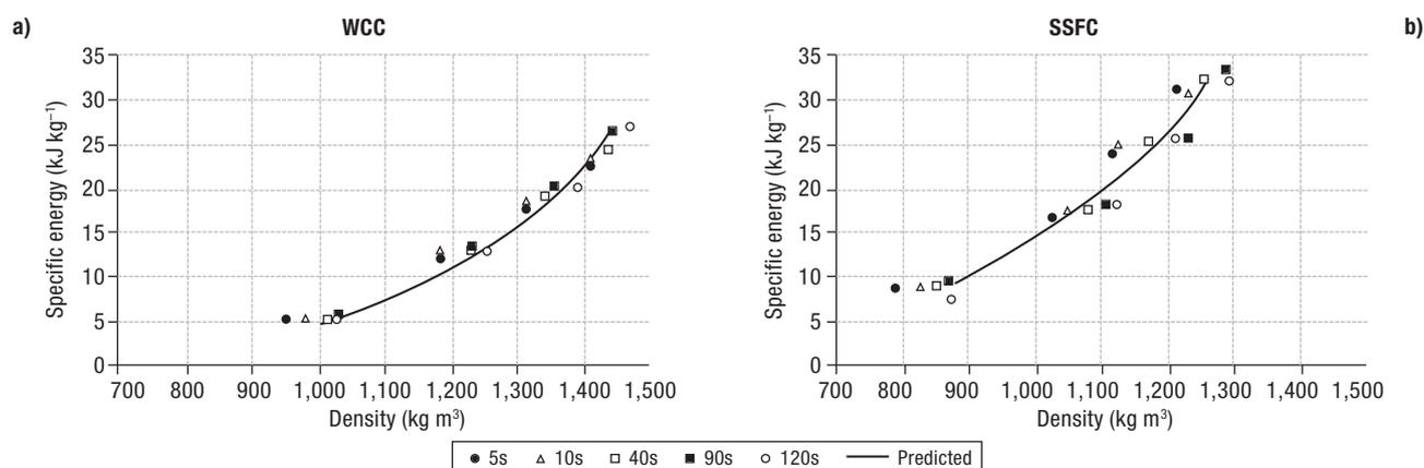
**Figure 7.** Relationship between specific compression energy and density to form the WCC (a) and SSFC (b) briquettes.
