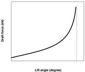
**Supplementary Figure 1.** A typical curve showing the predicted draft force against the lift angle, derived from an analytical model (*e.g.* Soehne's model and models derived from).
