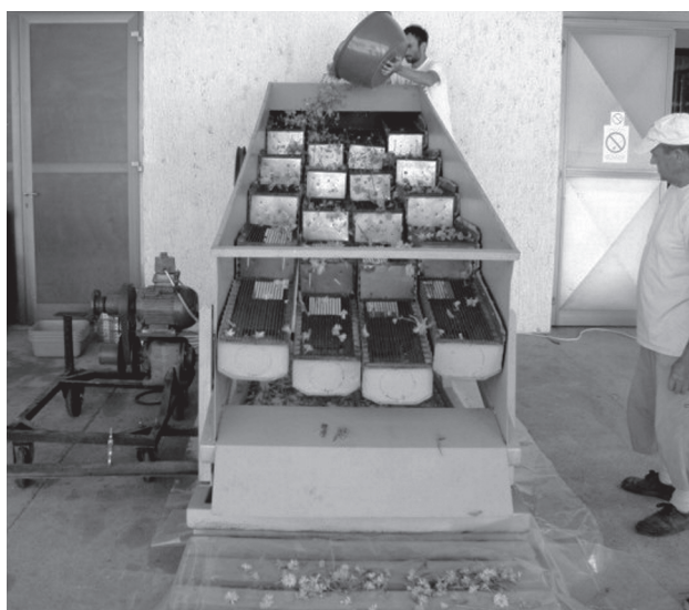
Figure 3. Device for separation of inflorescences from stalks and leaves
