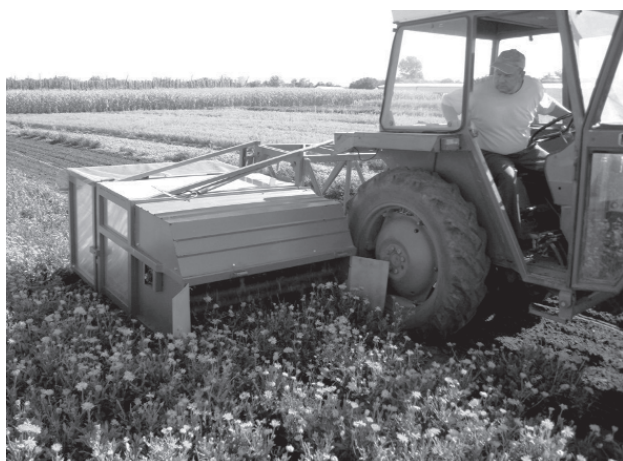
Figure 2. Tractor with mounted virtual rotating comb type harvester in the marigold inflorescences harvest
