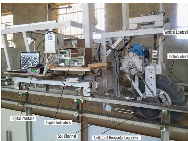
**Figure 1.** General testing facility setup and its components.
