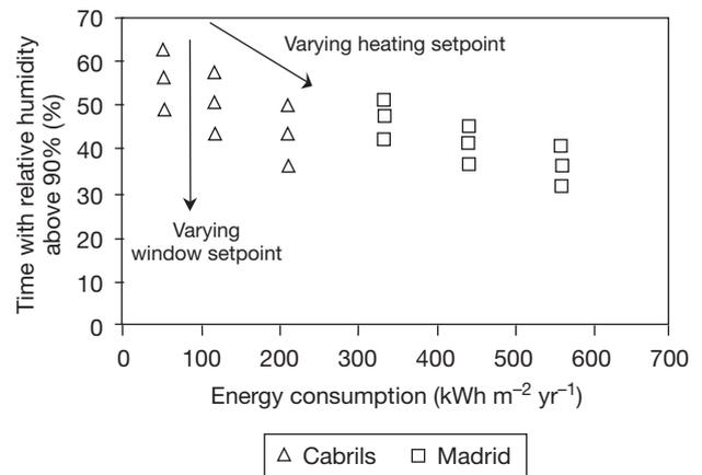
**Figure 1.** Results of the first set of simulations; relationships between energy consumption and period of high relative humidity (RH), varying heating setpoints (10/14, 12/16 and 14/18°C) and window setpoints (22/18, 24/20 and 26/22°C). The increase in heating setpoint strongly increased the energy consumption; the reduction in the window setpoint reduced the relative humidity. Each point is the average yearly value for one simulation strategy.
