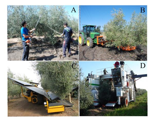
**Supplementary Figure S1.** Hand-held branch shakers removing fruits on nets (A); tractor-hitched trunk shaker on a high-density olive tree (B); side-by-side harvester detaching fruits using a trunk shaker and collecting them on a catch frame (C); and straddle harvester based on a canopy shaker collecting fruits on a catch frame (D).
