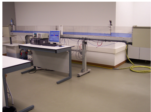
Figure 2. Prototype hydraulic canal in laboratory.
