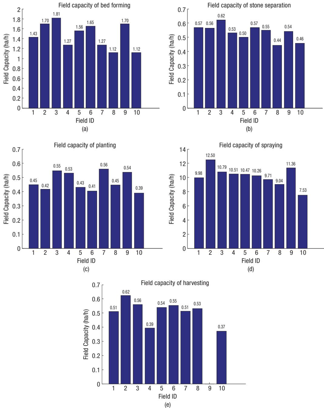
**Figure 7.** Field capacity distribution in bed forming (a), stone separation (b), planting (c), spraying (d) and harvesting (e).
