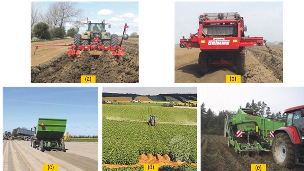
**Figure 1.** The involved field operations in potato production: (a) bed forming; (b) stone separation; (c) planting; (d) spraying (photo source: gopixpic); (e) harvesting.
