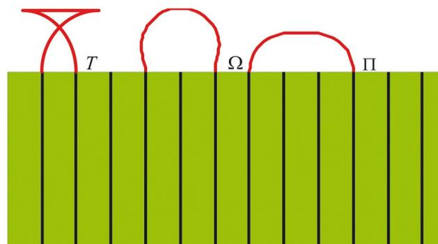
**Figure 5.** Three common types of turns  $T$ ,  $\Omega$  (skip 1 track), and  $\Pi$  (skip 2 tracks) used in bed forming.
