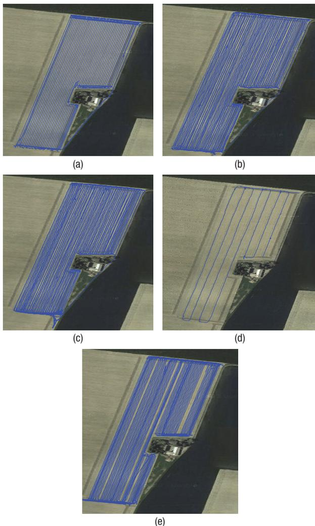
**Figure 4.** The GPS recordings for agricultural vehicles: (a) bed former, (b) stone separator, (c) planter, (d) sprayer, and (e) harvester in potato production in Field 3.
