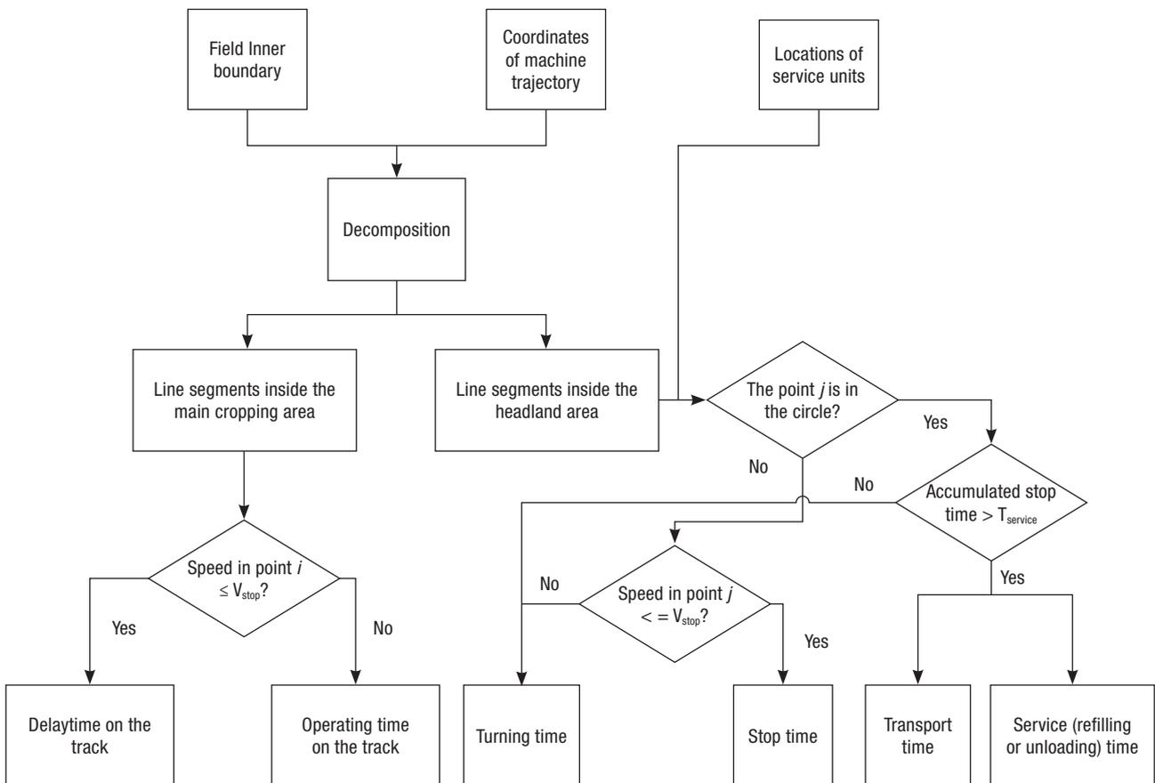
Figure 3. Flow diagram of the method of analysis of the recorded GPS data.
